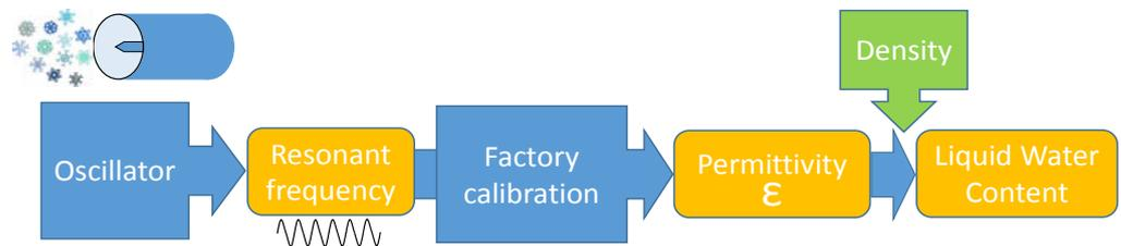
The measurement takes place in a sampler acting as a capacitor, where the electrodes are a metal cylinder and a central rod. Thanks to an internal resonator,  $WIS_{\epsilon}$  measures the resonant frequency of the system. This value is then converted into permittivity thanks to a conversion function determined at manufacturing time. In a second step, the permittivity is combined with the density of the snow (measured separately) in order to compute the liquid water content.
